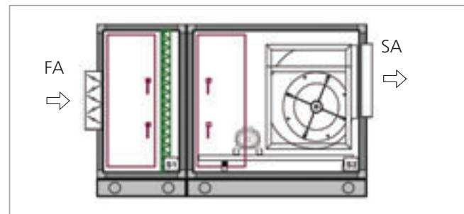
Filter chamber with damper and fan chamber is shown in Figure 1. The objective in this system is supplying the fresh air intake through a panel filter.
