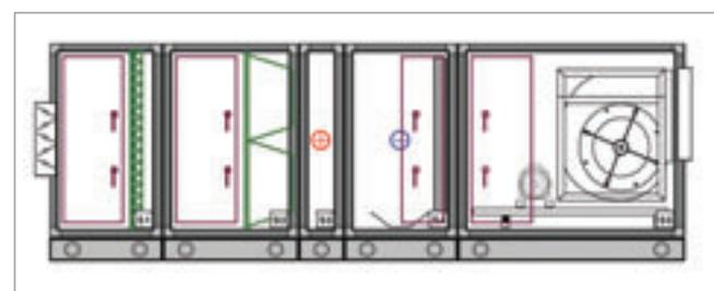
An air handling unit operating with 100 % fresh air is modelled in Figure 2. S2 chamber illustrates the bag filter and droplet retainers, and condensation pan is seen in S3 and S4 chambers along with the heating and cooling coils.
