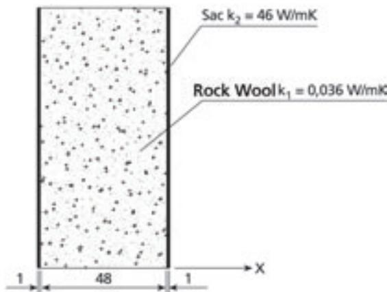
For example, we can calculate the heat conduction value by calculating heat conduction by taking the interior unit panel temperature as 17°C, the ambient temperature as 32°C for a surface area of 60 m<sup>2</sup>.
