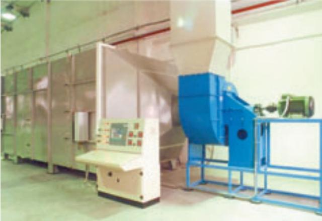
"Air Handling Unit Testing and Performance Measurement Room"
