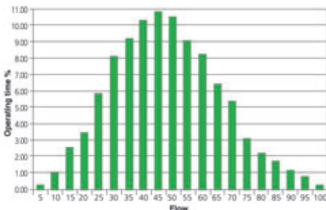
Air handling systems rarely need maximum design flow. Frequency converter alters the rpm of the fan motor in air handling units, adjusting the system air flow. In this way, while the required amount of fresh air is supplied, a high level of energy is saved. The following figure shows that 90% of the fan's operation occurs at 70% rpm.
