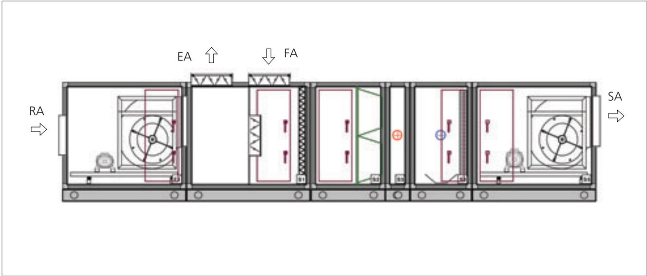
The design in Figure 3 is an air handling unit operating with mixed air. S1 in this figure shows the mixing chamber. This chamber determines how much of the intake air from the system is to be exhausted and how much to be added to the mixed air by working together with the dampers on it. These dampers can be controlled through servo motors governed by the automation system upon request. This allows comfort conditions to be ensured through minimum energy savings.
