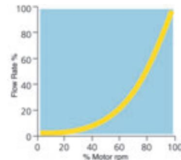
The most important point in terms of energy economy is that power consumption is proportional to the third power of fan rpm. This means that a drop in rpm will provide a significant reduction in energy consumption. Consequently, as seen in the figures as well, the power expended to bring the air flow to 75% is 40% of the energy of the motor operating at full speed.
