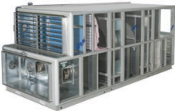
Double rotor air handling units are systems which provide high energy efficiency especially in conditions of high temperature and high humidity. For double rotor air handling units to operate with the expected energy efficiency, they should be operated without interruption with 100% or nearly %100 fresh air.
