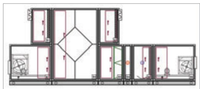
drainage pipe (stainless steel) of this pan is hermetically extended outside the unit. It is hygienically important to mount a filter outside the filter on the intake side and before the heat recovery coil on the exhaust side.
