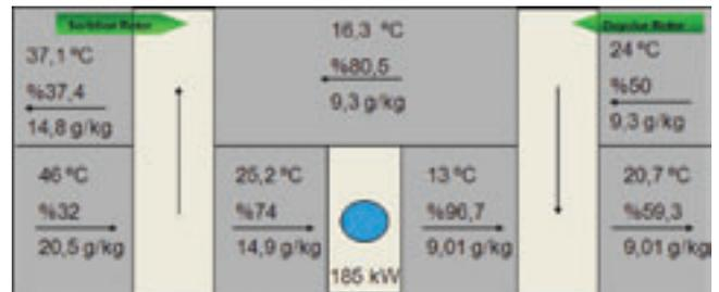
Double Rotor Air Handling Units Design Values
