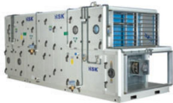
Interior and exterior surface material: Interior and exterior surface sheets have been manufactured from galvanized steel sheet. The exterior sheet surface is coated with 5 μ epoxy prime coat, a 20 μ polyester furnace paint top coat with colour code RAL 7035 and plastic film over the paint. Interior and exterior sheet thicknesses can be selected within the range 0.8 - 1.2 mm depending on requirements and place of use.
