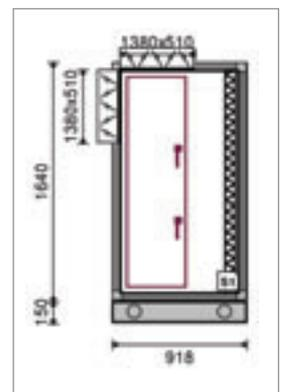
The three-way mixing chamber has been designed for similar purposes. However, this system includes a fan for return air and while the desired portion of return air is given back to the system, the remainder can be exhausted.
