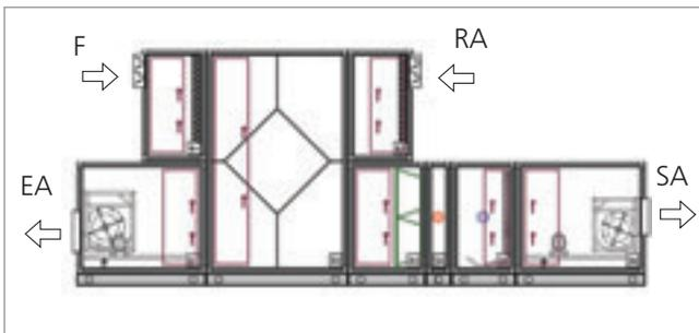
Air handling unit with heat recovery is shown on Figure 4. Heat recovery unit [S2] supplies the intake heat from the exhaust air to the fresh air and considerably increases the system efficiency.
