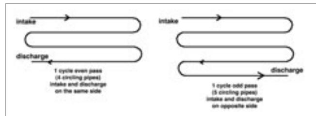
Figure 3.4. Intake - Discharge Directions According to Odd or Even Numbered Passes in Water Side Coil
