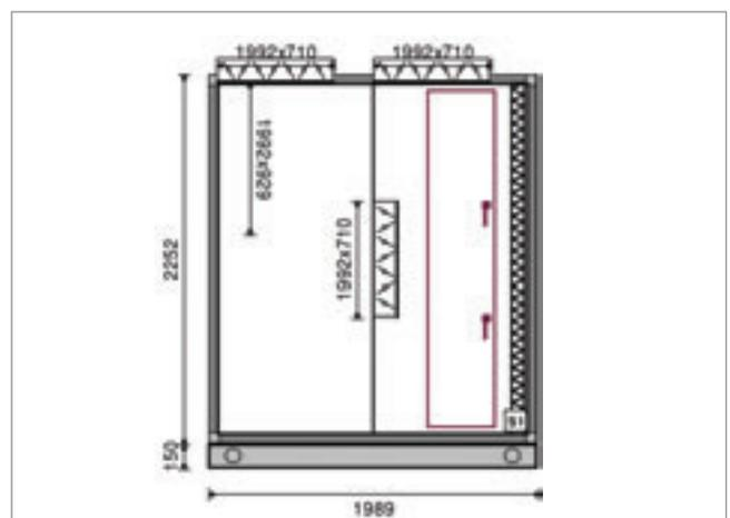
Dampers used on both types of mixing chambers have opposing blades and have been designed to allow them to be controlled individually.
