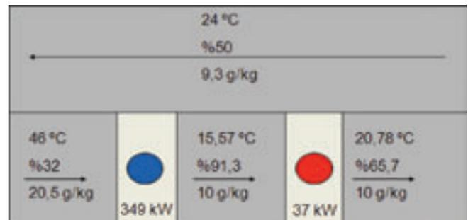
Design Values for a 100% Fresh Air Air Handling Unit without Heat Recovery
