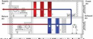
Night Operation Where Dehumidification Is Applied: Dehumidification is realized in the night operation with low usage by having the air of the location pass through the heat pipe and evaporator. The cool air coming out from the evaporator with condensed moisture passes through the heat pipe (upper part) and the condenser, and is sent to the pool location heated. (The air can be further heated up by initiating the final heater if necessary)
