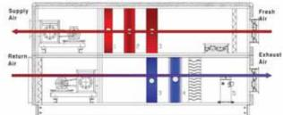
Operation During Season Changes: (Dehumidification ON/ OFF) Dehumidification and ventilation process is done with a maximum fresh air volume. (A great part of the circulating air is discharged to the outside environment)
