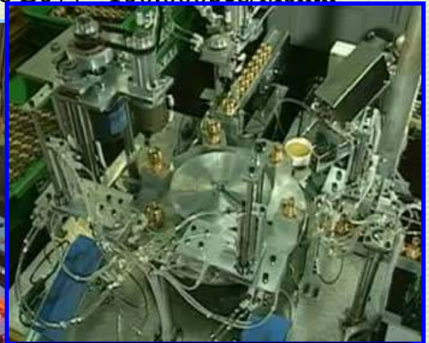
Automatic Assembling Machine of the Fittings for PEX, ML
