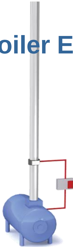
Boiler exhaust with over-draft control
